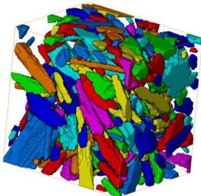
Figure 6 - 3D reconstruction of the sunflower aggregates within the metakaolin binder paste
