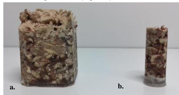
Figure 2 - Sunflower-based samples (a) prismatic sample with a base of 2.33 x 2.33 cm<sup>2</sup> and (b) cylindrical sample with a diameter of 8.8 mm.
