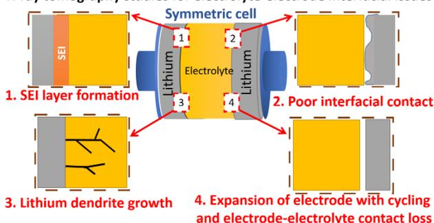
Figure 1. Schematic presenting application of X-ray tomography to understand the interfacial contact phenomena in solid-state Li metal batteries.
