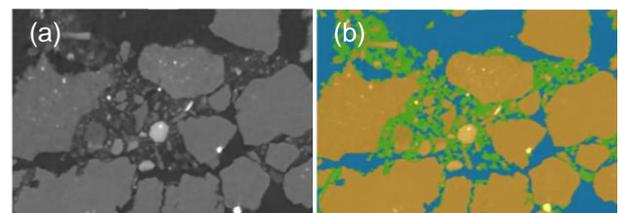
Fig 1: Original (a) and segmented (b) slice showing grains (yellow), water (blue) and deposits (green).
