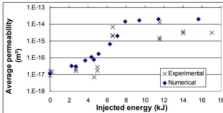
Figure 5 - Comparison of the experimental and the numerical average permeability under high confinement with variable injected energy.
