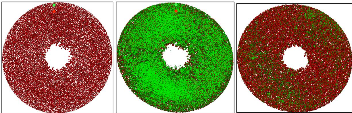
Figure 11- Xray images for scanned fractures at 18µm resolution: clean fracture (left), clogged fracture (middle), unclogged fracture (right). Particles in red are proppant particles, particles in green are crushed sand particles.
