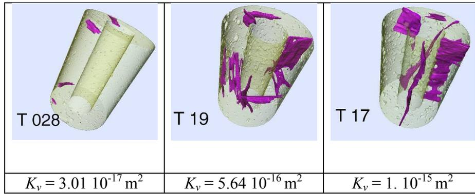
Figure 3 - 3D tomography scans after one shock (left), three shocks (middle) and nine shocks (right). Tests under high confinement.
