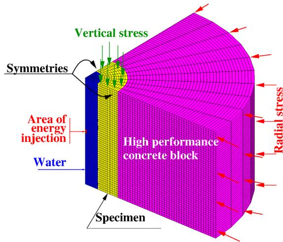
Figure 4 - Finite element model of the simulation of tests on hollow cylinders.
