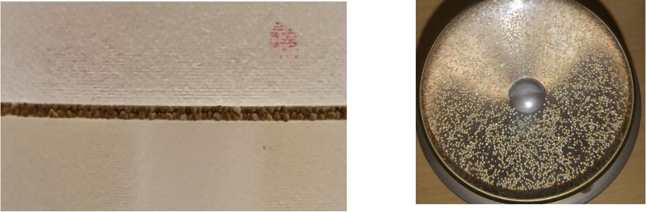
Figure 7- Left: Side view of a fracture filled with 2 layers of proppant; right: top view of a fracture filled with 0.5 layer.
