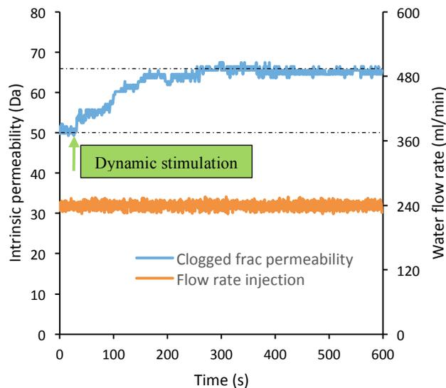
Figure 9- Permeability evolution after applying a dynamic load on a clogged fracture with 0.5 layer of proppant.
