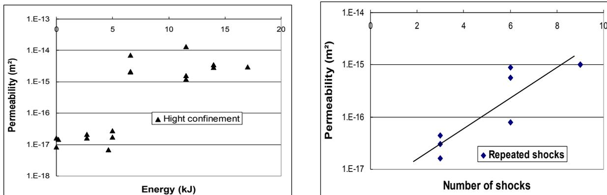
Figure 2 - Evolution of the permeability with injected electrical energy for a single shock on mortar specimens (left), and for repeated shocks (right). Tests under high confinement.
