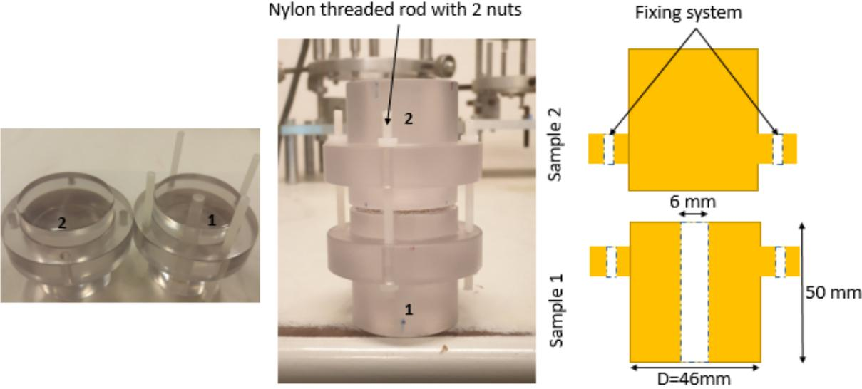
Figure 6- Polycarbonate samples details.
