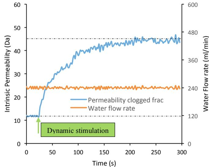
Figure 10- Permeability evolution after applying a dynamic load on a clogged fracture with 2 proppant layers.
