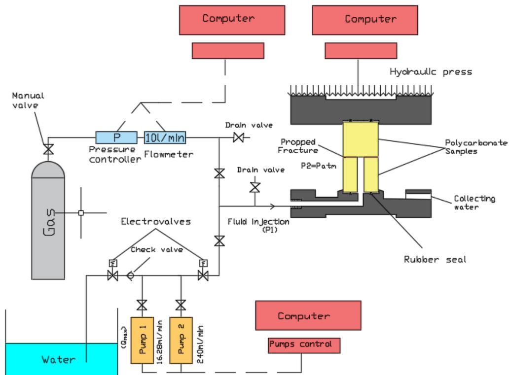
Figure 8- Schematic of the complete experimental apparatus.
